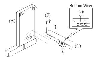
1. Insert the Adjuster (G) on the bottom of Pedal Board (C). Fasten Side Panel (A) and Pedal Board (C) with four bolts (F).
